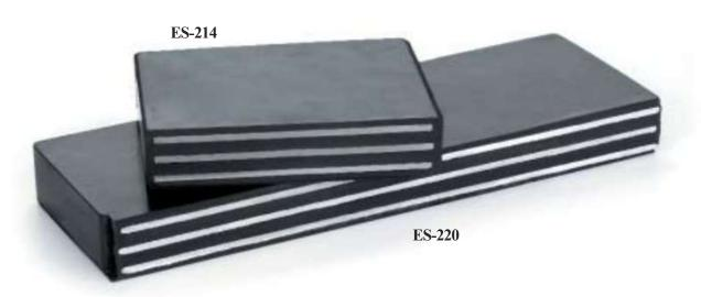
The layering of sound non-absorbent (e.g. metal) and sound absorbent (e.g. rubber) materials results in additional reflection damping (see page 31). With a low degree of deflection, the layer achieves the best possible degree of damping for the smallest possible compliance. Layers are suitable for loads of 300 to 800 N/cm2.
