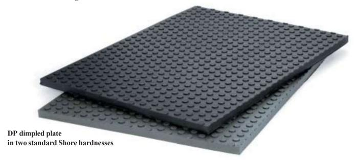
The dimples on the damping plate have a simple but effective function: They reduce the supporting surface area. This increases the deflection/damping effect. The dimples provide support up to the specified load. Thereafter, they are completely compressed and damping takes place as before as a plate with a flat surface. This system enables improved damping values and provides additional loading security since it is practically impossible to overload the plate.
